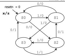
$$\begin{aligned} Q_1(t+1) &\leftarrow \overline{(Q_1+Q_0) \oplus x} \\ Q_0(t+1) &\leftarrow x \overline{Q_1} + Q_1 \overline{Q_0} \\ z &= \overline{x} Q_1 + Q_1 Q_0 \end{aligned}$$
