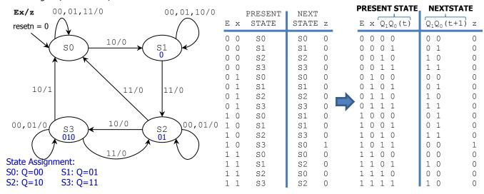
This is a Mealy Machine. The output z depends on the input as well as on the present state.
