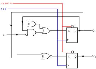
$\checkmark$  Complete the timing diagram.  $Q = Q_1 Q_0$  (Tip: get the excitation table) (6 pts)
